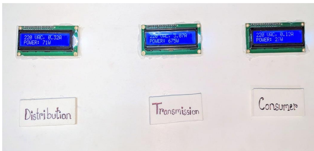
Figure 5.2.2.1: Display of the system
