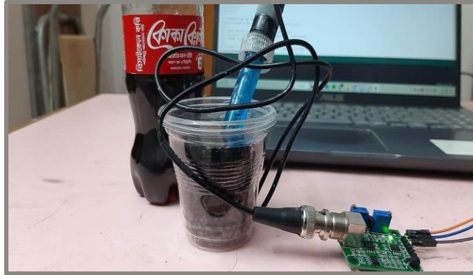
Fig. 5.2. pH sensor calibration with coke
