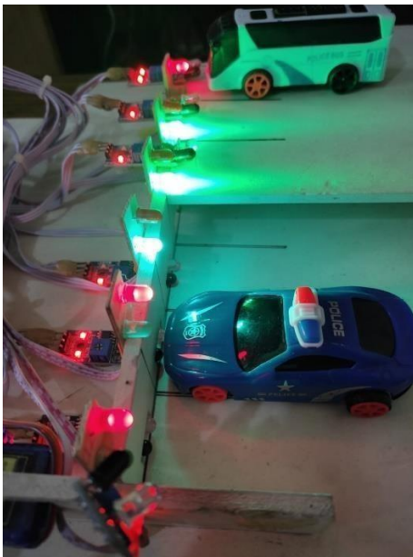
Figure 25: LED turn red at the booking spot & the website shows the slot is full
