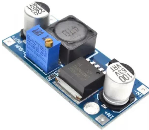
Fig. 3.9 DC to DC Buck-Converter
