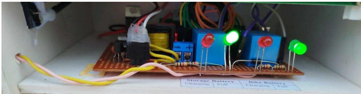
Fig. 5.2.5. Right side Green light is on while charging is complete.
