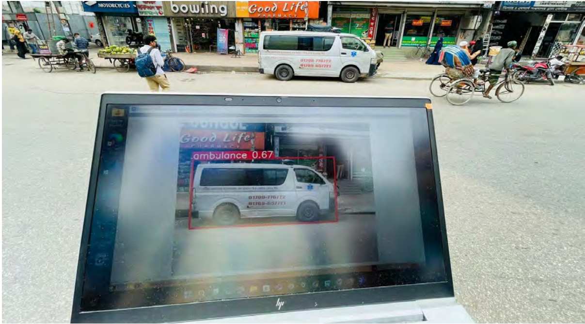
Figure 39: Emergency Vehicle detection In Real Life
