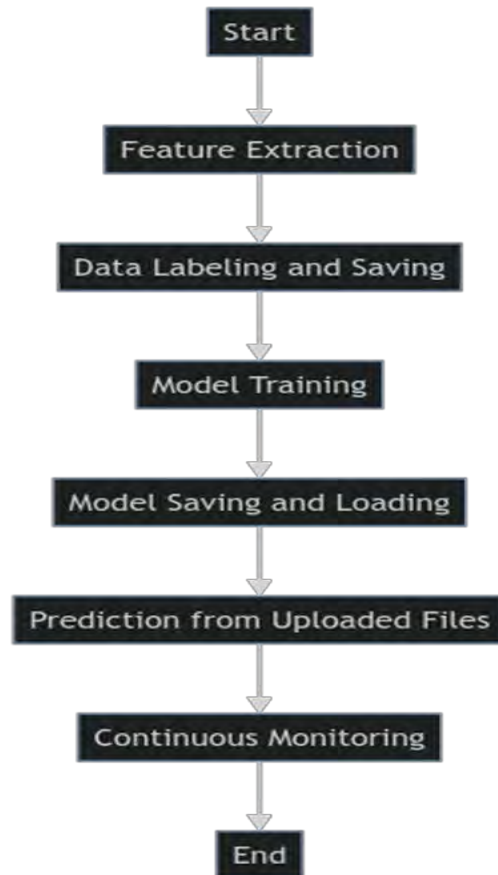
Figure 27: Program flowchart for the LSTM Model
