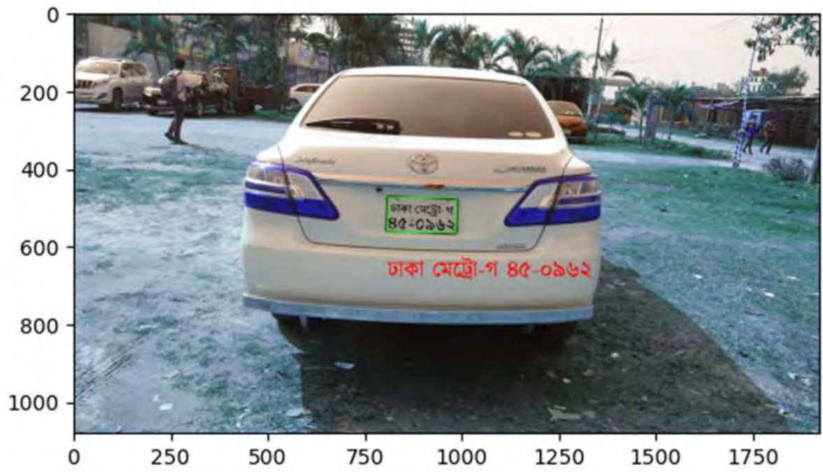
Figure 19: The output from the captured picture after number plate detection.
