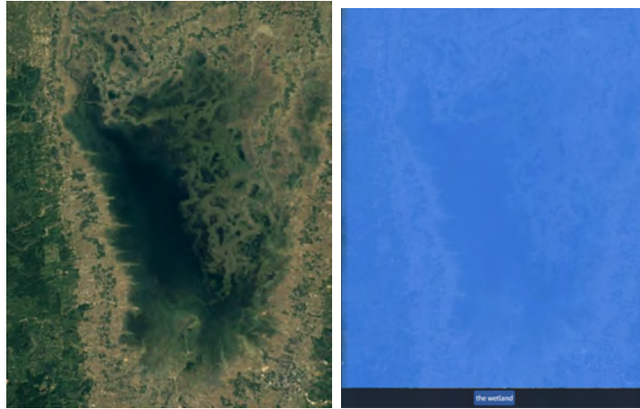
Figure 5.2: Segmentation of PaliGemma on Satellite Image. The prompt was given 'segment the wetland'. The model used was paligemma-3b-mix-224 with greedy decoding.
