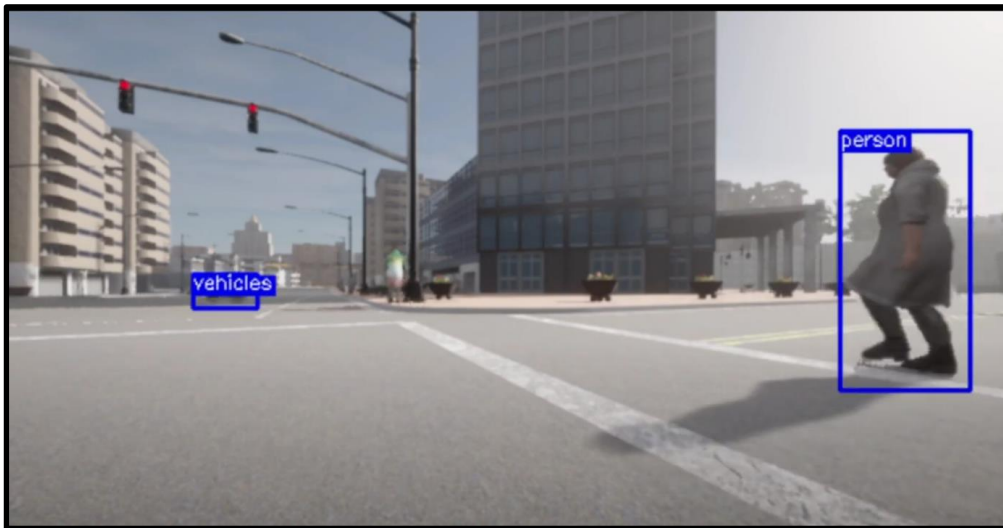
Fig 42: Vehicle stops, keeping a minimum braking distance between it and the front person
