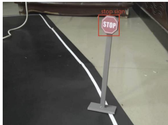
Fig 70: Vehicle detecting stop sign ahead with bounding box width of 90 pixels
