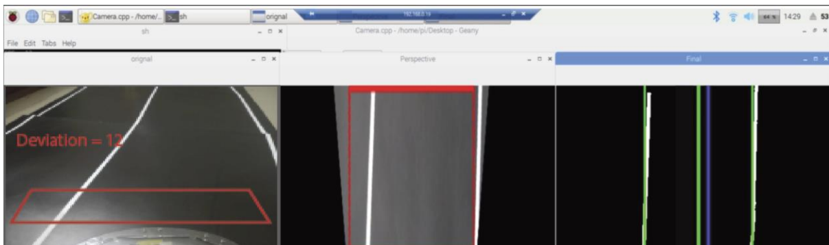
Fig 61: Vehicle having a difference of 12 units between its frame center (blue) and lane center (green)
