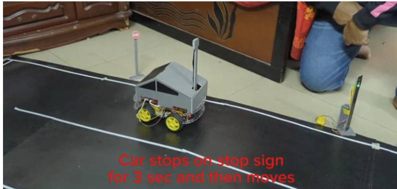
Fig 71: Vehicle detecting stop sign ahead and decides to stop for 4 seconds before moving on for 1 second
