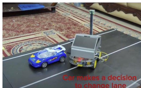
Fig 66: Vehicle detecting car ahead within 5 to 30 cm and changing lanes to the left
