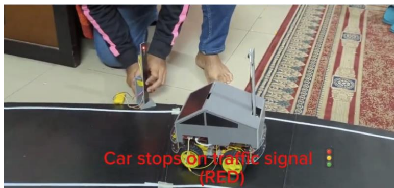
Fig 68: Vehicle detecting red traffic signal ahead within 5 to 20 cm and decides to stop
