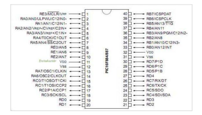
Fig 2.4: 40 Pin PIC16F887 pin Assessment
