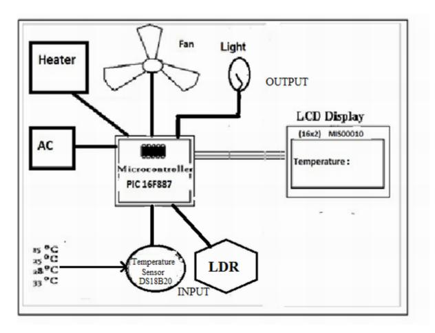
Fig 3.2: Block Diagram of Smart Appliance system
