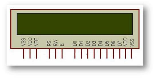
Fig 3.6: LCD Model MIS00010
