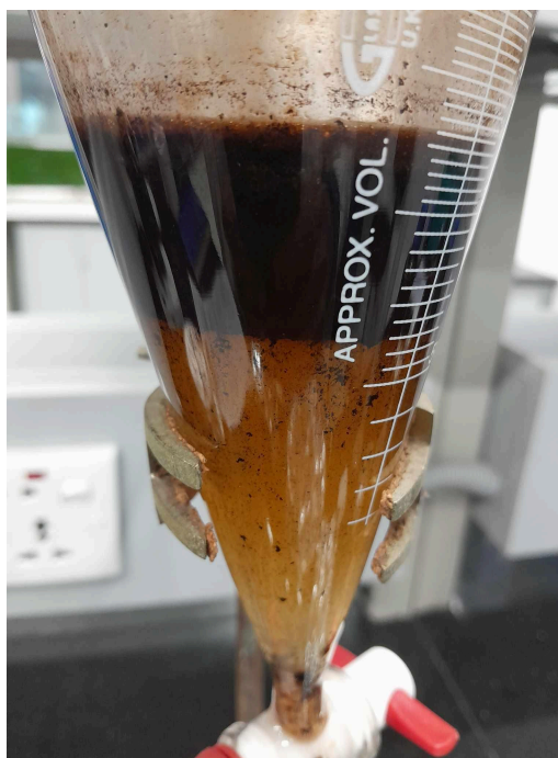
Figure 2.2: Solvent-solvent partitioning of bark of Holarrhena pubescens
