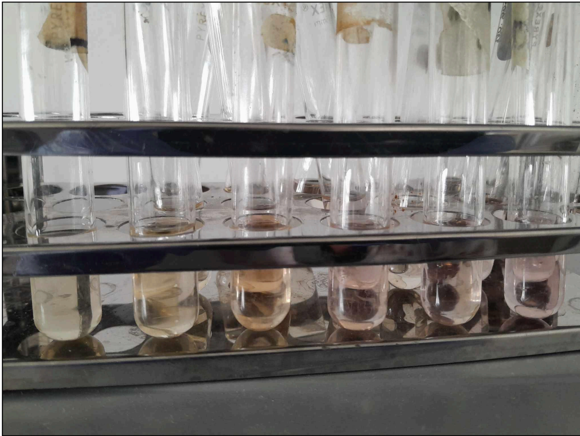
Figure 3.6: Change in color of DPPH due to antioxidant activity, purple to yellow
