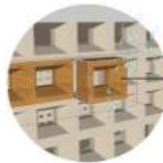
45 DEGREE ANGLE ON THR BRICK ACTS RAIN AND DIRECT HEAT.
