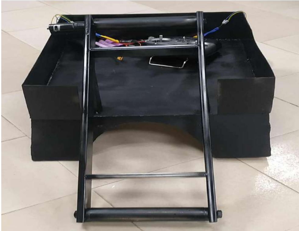
Figure 23: Frame of the Aqua Rover
