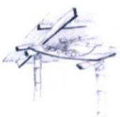
STORAGE INSIDE THE ROOM, SUPPORTED BY BAMBOO STRUCTURAL MEMBERS, USED AS STORAGE SPACE.
