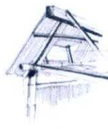
PUNCH CUT OUT FROM SLANTED TIN ROOF. IT IS USED AS AN OPERABLE WINDOW TO REGULATE LIGHT AND VENTILATION.
