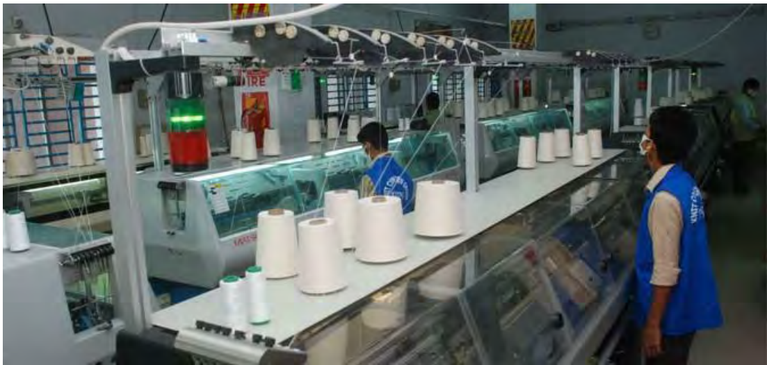
Fig 2.3: Flatbed knitting machine
