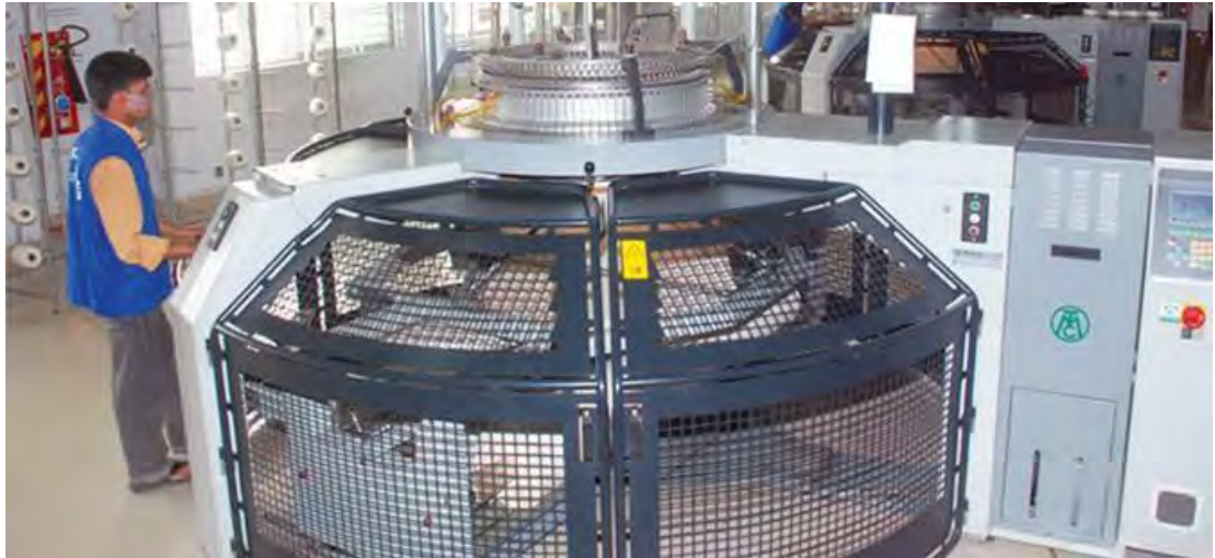
Fig 2.2 Circular knitting machine
