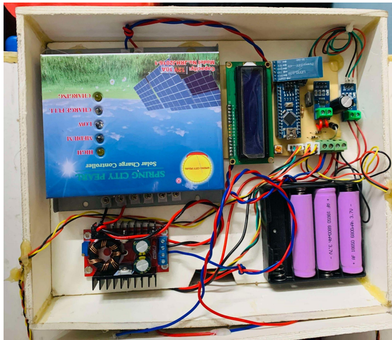
Figure70 :Electrical circuit and component box of prototype
