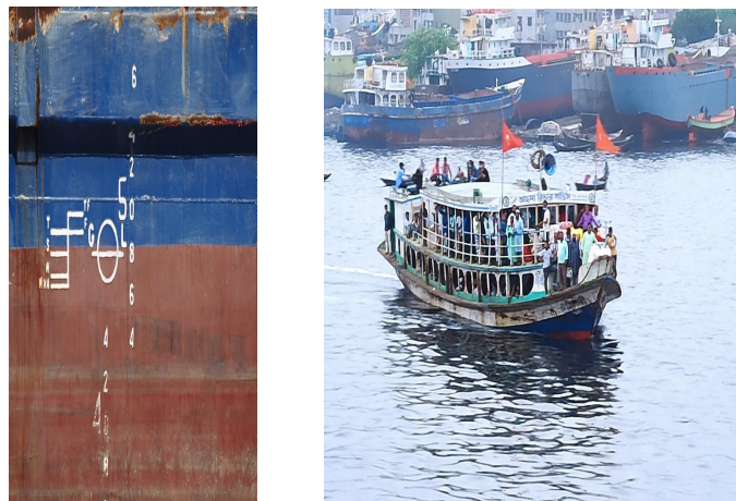
Figure 6.3: Load line image
