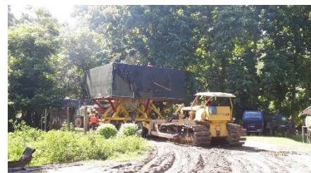
Figure -10 Transportation of Heavy Materials (Runner)
