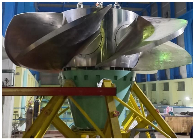
Figure - 3 Complete Runner with Cone at Site
