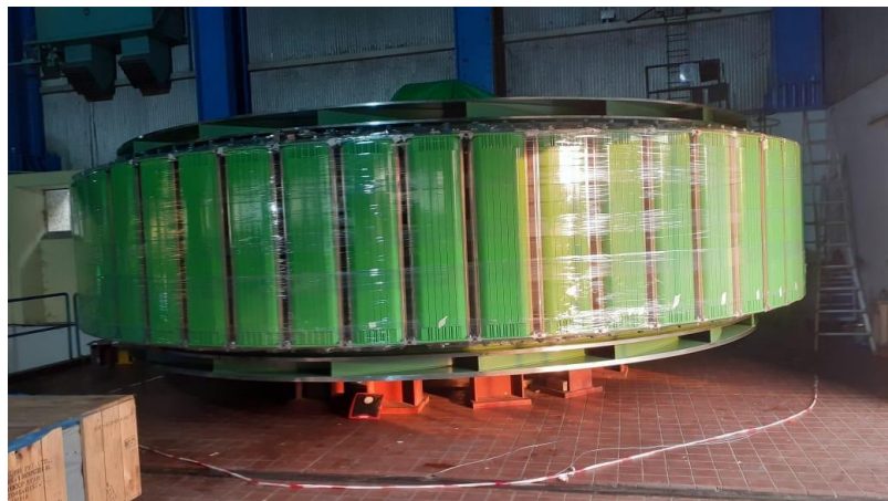
Figure-7 Rotor With field Pole
