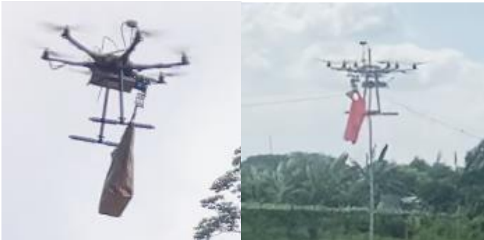
Figure: Payload is being carried with Mechanical Claw
