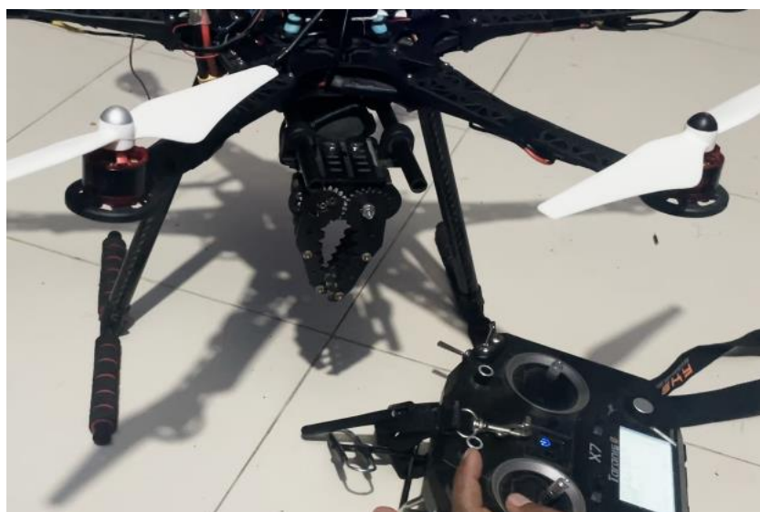
Figure: Controlling Mechanical Claw with Radio Controller
