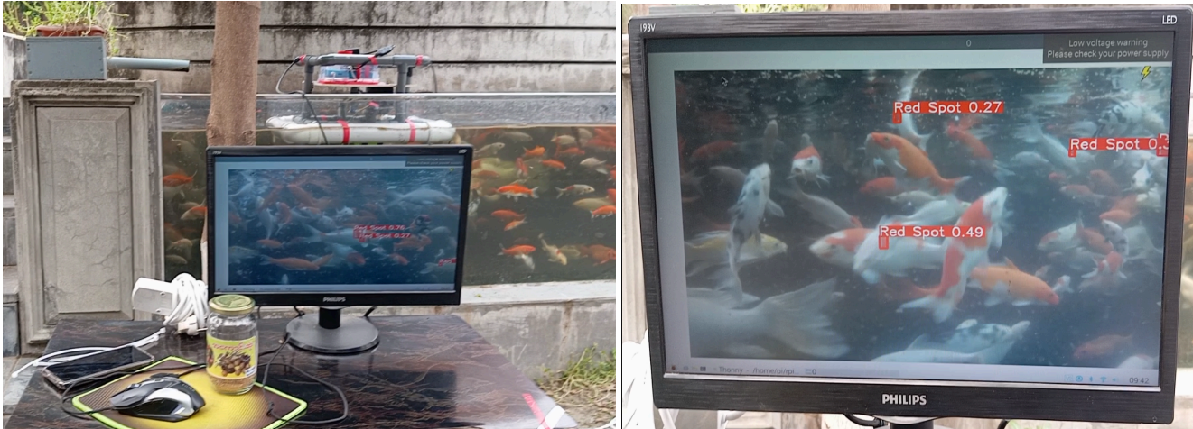
Fig 3.3: Monitoring the presence of spotted fishes (Red Spot/EUS) in an indoor fish farming system and displaying the information on a monitor.
