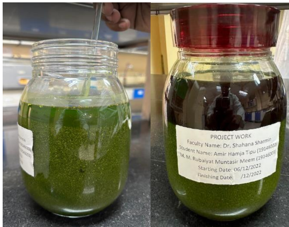
Figure 2.4: Approximately 1L Ethanol mixed with the powder for extraction.
