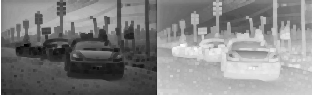
Figure 5.2: Dark Channel Image and Transmission Map Forecast Image
