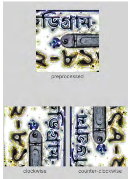
Figure 3.1: 90 degrees rotation augmentation
