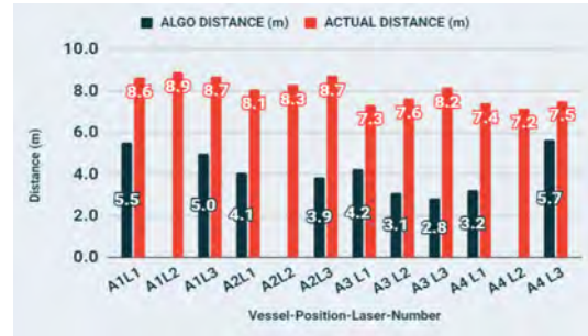
(b) Vessel A's Lasers' Distances at 4 Positions
