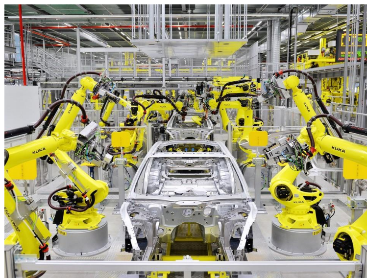
Figure 13: Passenger vehicle body welding through robots in body shop.
