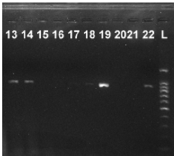
Figure 4.6: Agarose gel showing specific bands for VP4 gene visualized in 1.5 % agarose gel with gel red staining. Sample 13, 14, 18, 19 and 22 are positive samples of amplified VP4 gene.
