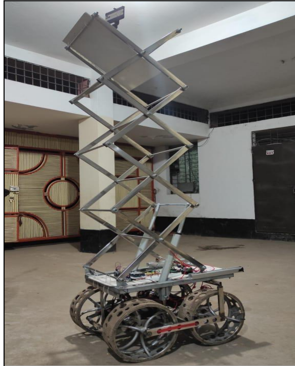
Figure 33: Scissor Lift while expanding (7 feet)
