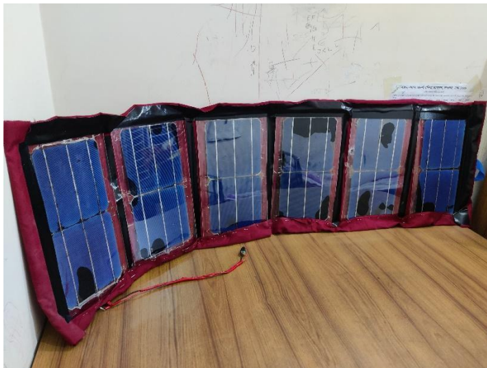
Figure 35: Portable solar panel setup
