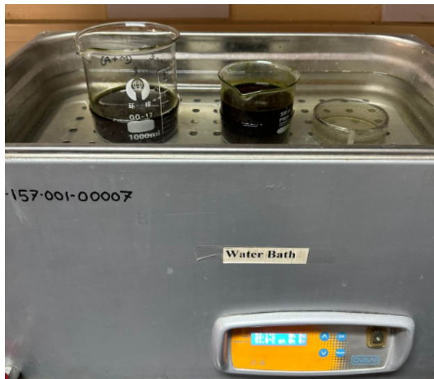
Figure 2.7: Evaporating Solvent from the Extract Using Laboratory Water Bath
