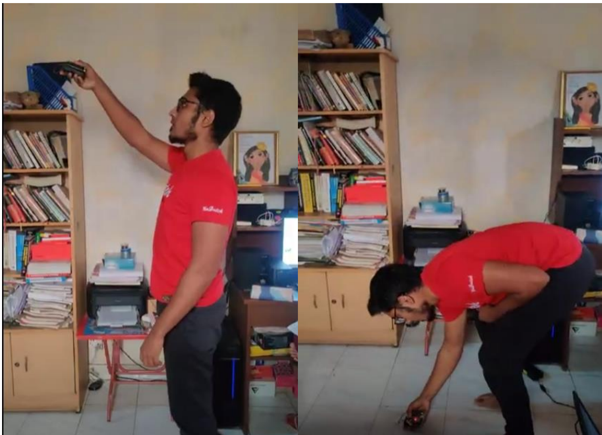
Figure 24. Dropping MPU6050 sensor from a height
