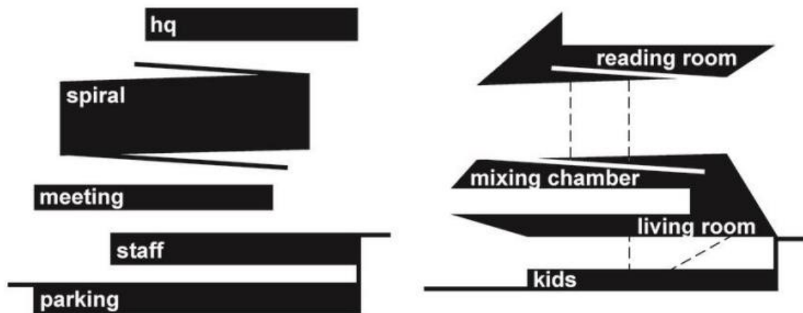
Fig 4.3.2:vertical zoning of the library building (five stable platforms and four unstable platforms). Source: Architect Joshua Prince-Ramus the first American to claim the $100,000 Marcus Prize. (2018). Archpaper.com. Retrieved 11 March 2018, from https://archpaper.com/2015/09/architect-joshua-prince-ramus-claims-100000-marcus-prize
