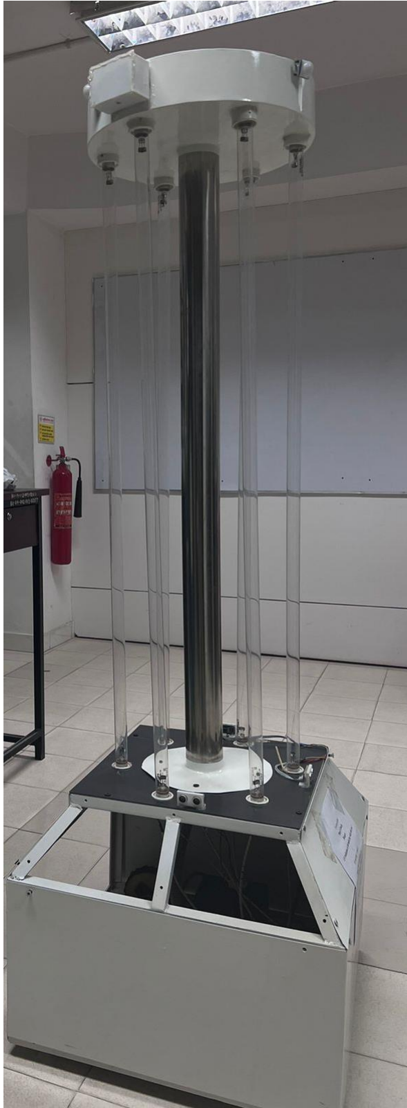
Figure 27: Mechanical part of the disinfecting system after sensors setup.
