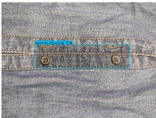
Figure 5.4: "missing button" class test image result
