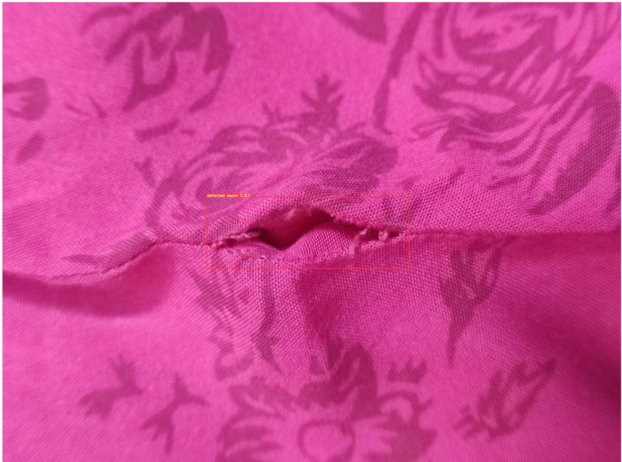
Figure 5.11: "defected seam" class test image result after 300 epochs
