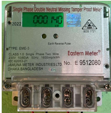
Figure-34: BSTI certified Energy meter
