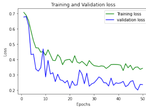
Figure 7.8: Training loss and Testing loss of ResNet152
