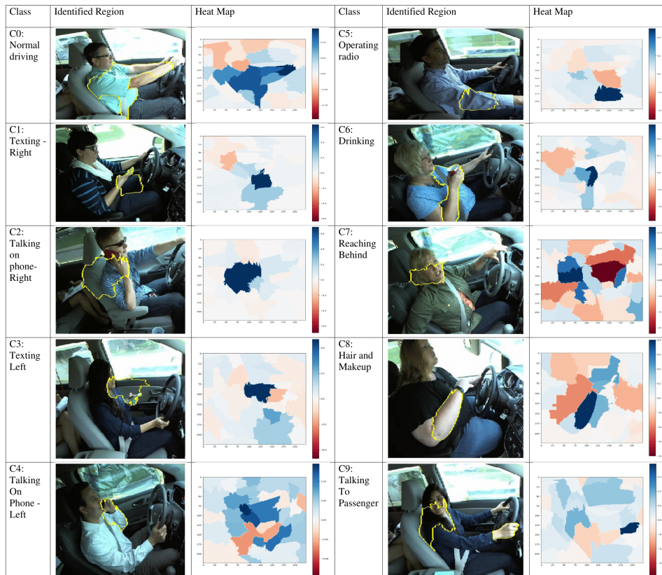
Figure 6.13: 6 layer CNN ROI Identification in SFD3 Dataset
