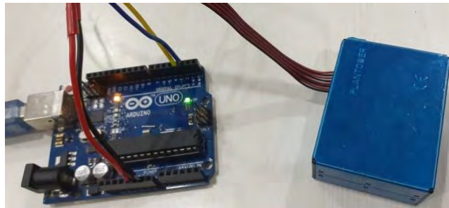
Figure 3.8: Real-time PM2.5 AQ sensor connected with Arduino [22].
