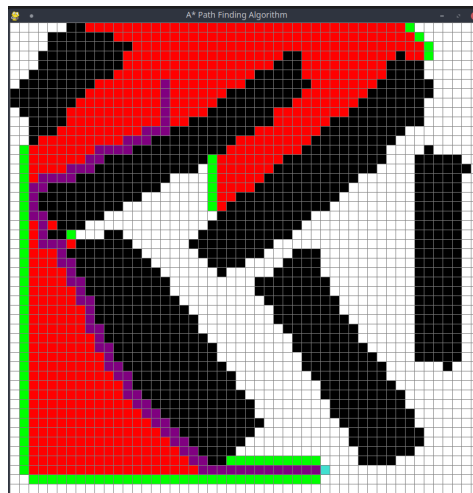
Figure 4.7: Shortest path using A* algorithm of plant bed configuration 2
