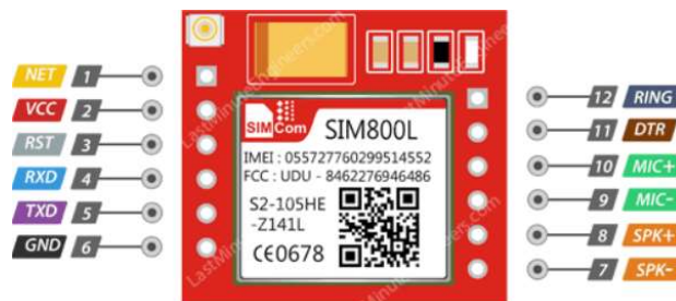
Fig 41: GSM Module SIM800L pinouts
