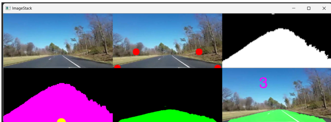
Figure 8.8: Complete process of lane detection
