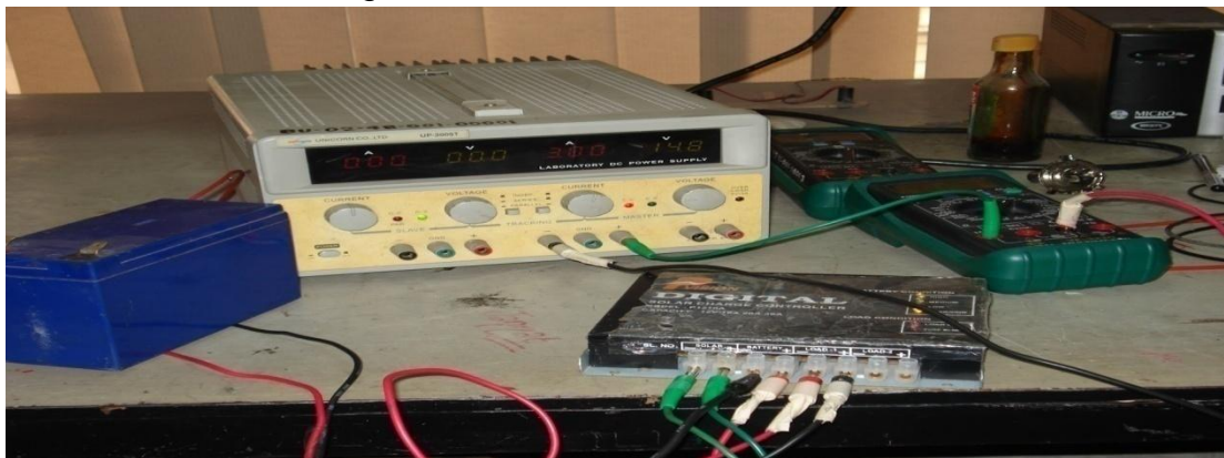
Figure8.1: Off load test
