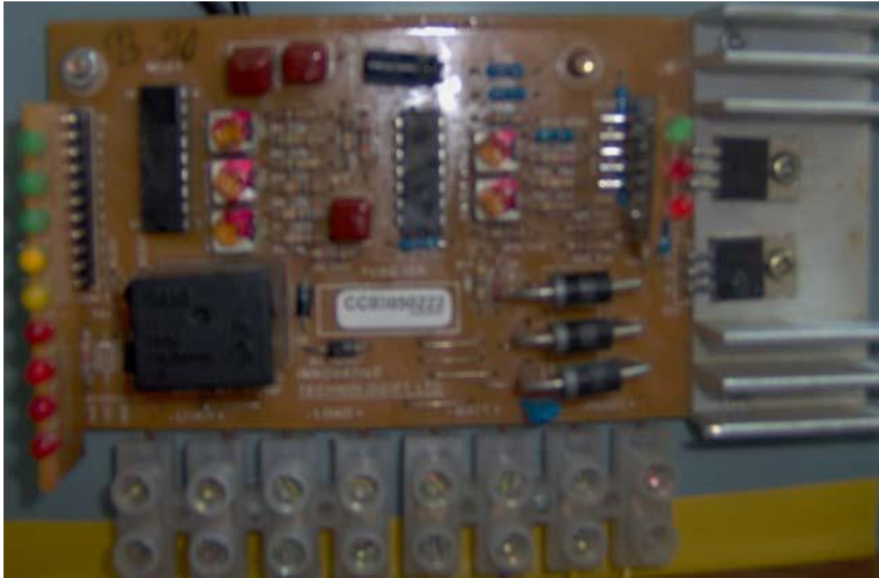
Figure8.5: Circuit of the Rahimafrooz charge controller
