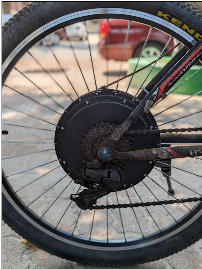
Figure 54: Mounted hub motor in the wheel
