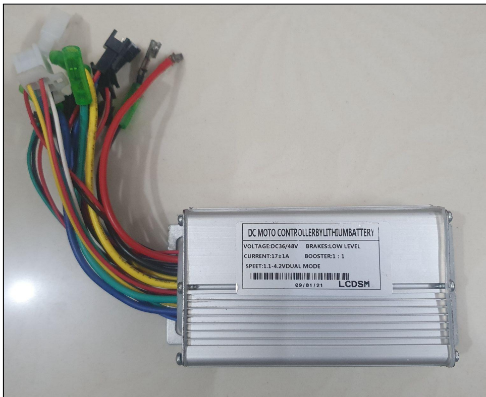
Figure 46: BLDC motor controller (secondary). Ratings: 36/48 Volts, 17±1 Ampere.
