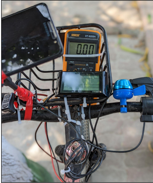
Figure 53: Multimeter and tachometer placement
