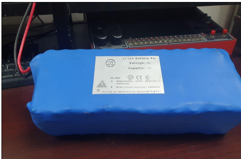
Figure 44: The main battery of the bike. Rated voltage- 48V and rated current- 10Ah.
