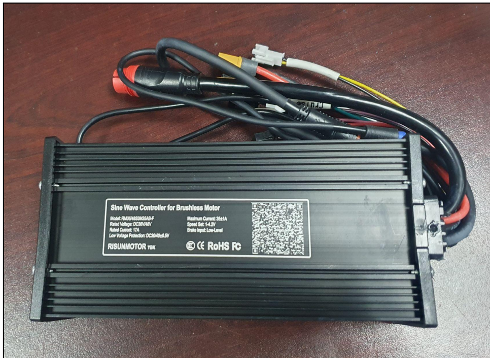
Figure 45: BLDC motor controller. Ratings: 36/48/72Volts, 17Ampere.
