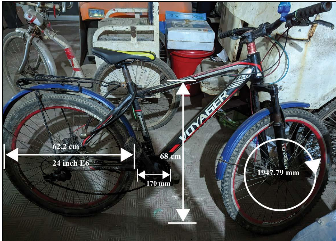
Figure 42: Prototype e-bike for conversion
