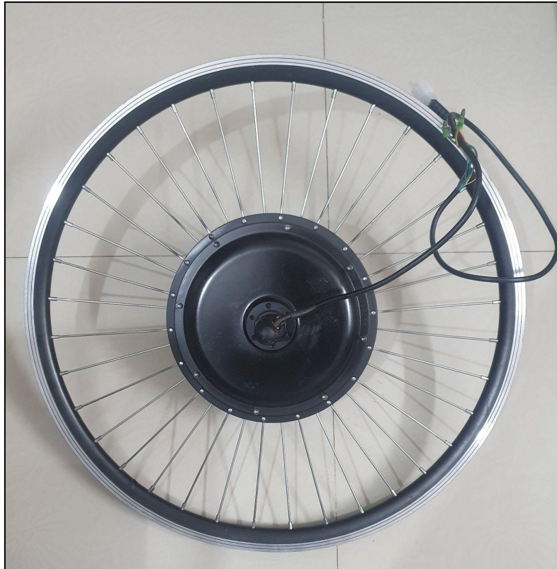
Figure 43: Wheel of the bike with the hub motor.
