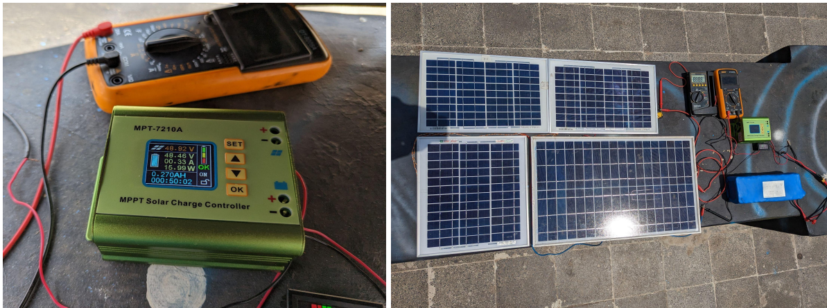
Figure 62: MPPT solar charge controller result at 50th minute and backup system construction
