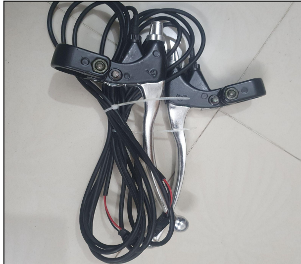
Figure 47: Electric brakes of the bike
