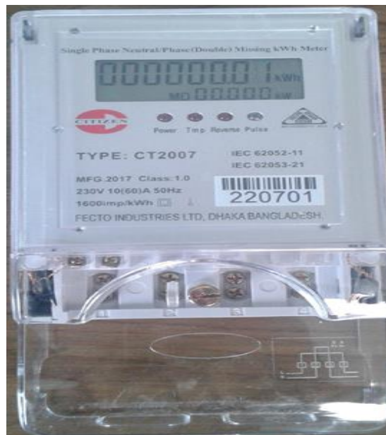
Fig. A.1 Electrical energy meter.
