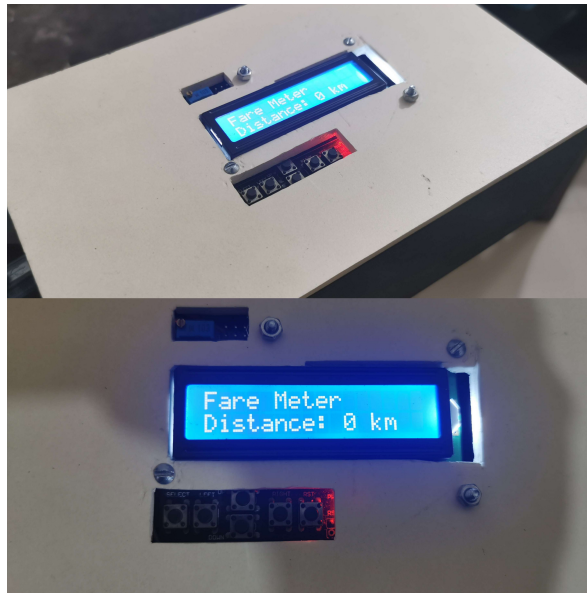
Figure 6.6: System in a Chassis ready to be mounted on Rickshaw
