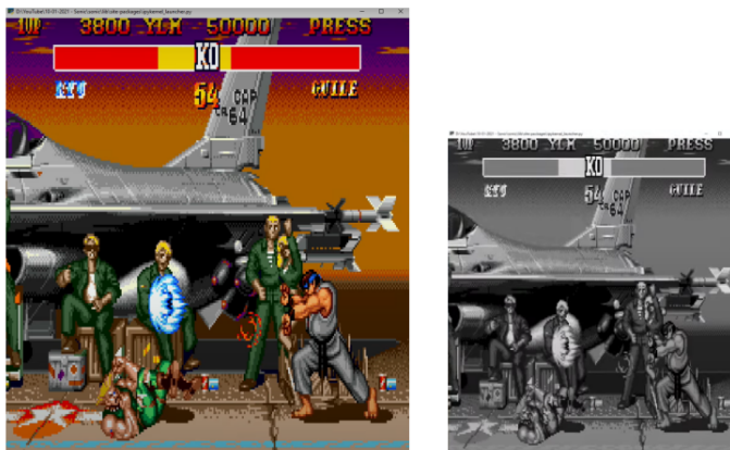
Figure 3.1: Gray scaling and reshaping of a frame to drop pixels
