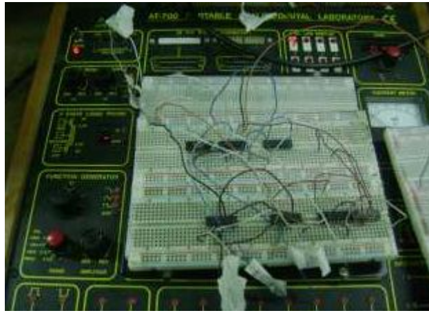
Fig: 3.7 Hardware implementation of Door security system
