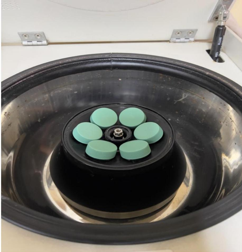
**Fig 3.6: 50ml falcon tubes in centrifuge machine**
