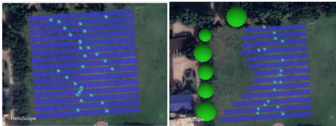
Fig. 3.7 Design layout of solar PV system without and with shading effects. The green circles represent nearby trees overshadowing the system.
