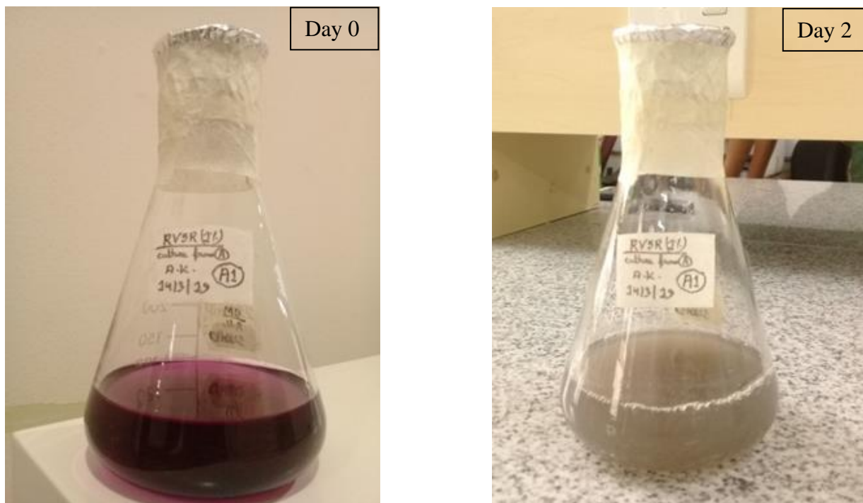
Figure 8: 4th flask A1 (directly inoculated from flask A after complete decolorization within 2 days). From right to left - inoculation day (day 1), after 48h (day 2).
