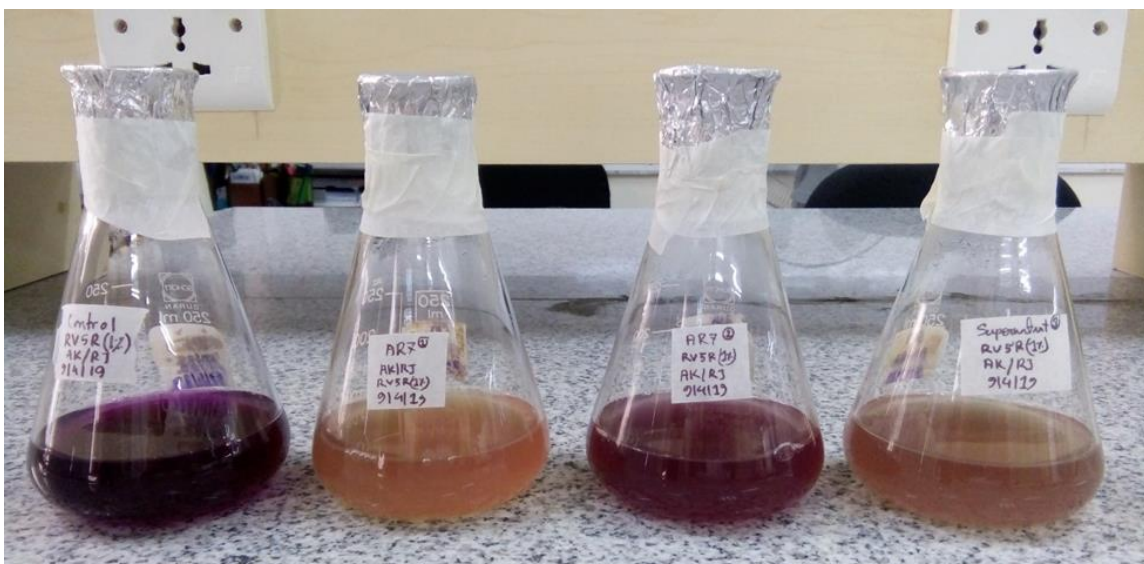
Figure 13: Dye decolorization of AR7 isolate after 24 hours (day1). The 1st flask from the right contains the supernatant as inoculate.
