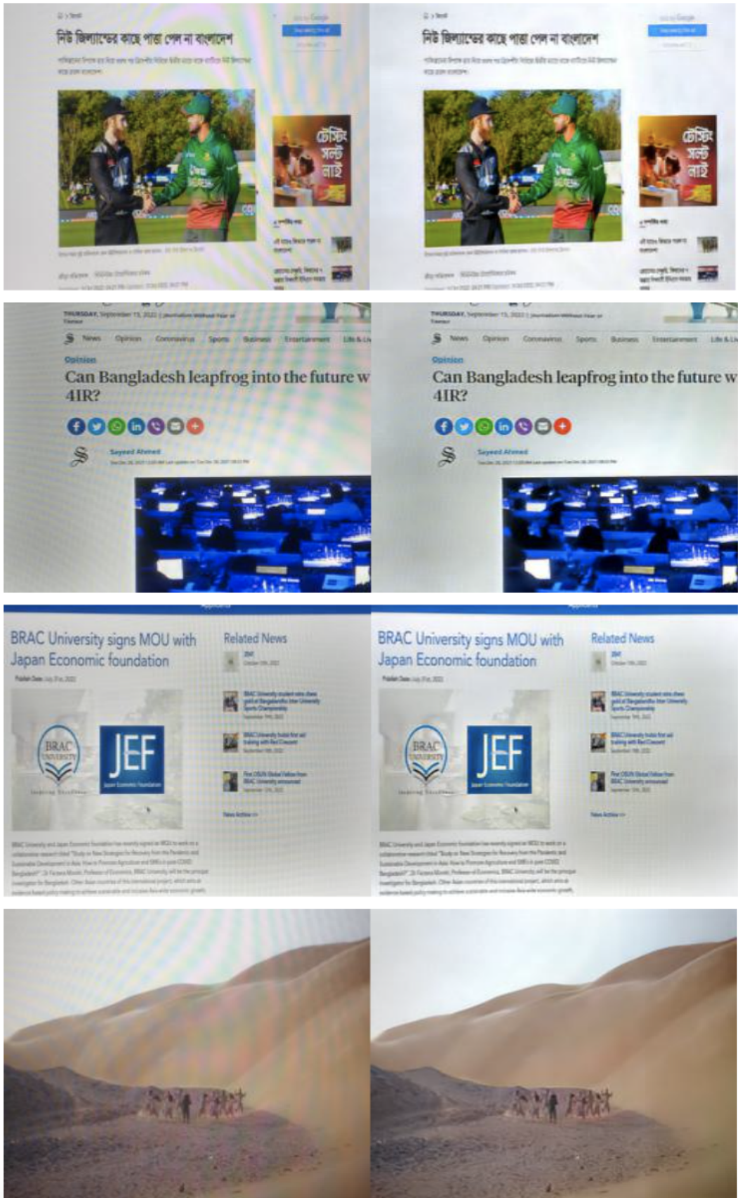
Figure 5.3: Restoration of screen captured moiré photos taken with Motorola Moto G3
