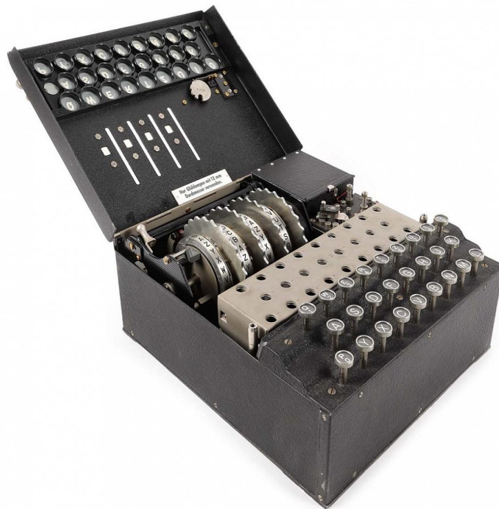
Figure 2.2: The Enigma machine
