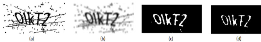
Figure 4.4: (a) gray scale image (b) blurred image (c) thresholder image and (d) eroded image
